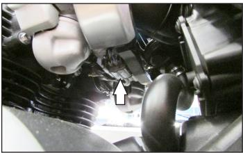
9 Plug the PC6 in-line of the TPS and wiring harness.
