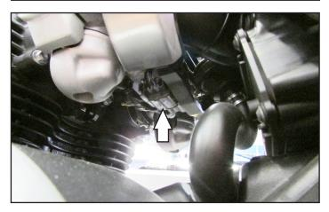
14 Plug the PC6 in-line of the TPS and stock wiring harness.
