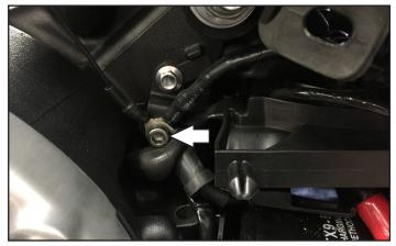
Route the PC6 harness along the left side of the air box and go up towards the backbone of the frame.
