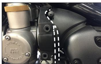
13 Unplug the stock Throttle Position Sensor connector.
