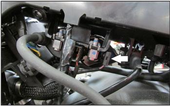
12 Unplug the signal wire of stock wiring harness from the #2 ignition coil.
