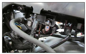
17 Unplug the signal wire of stock wiring harness from the #2 ignition coil.
