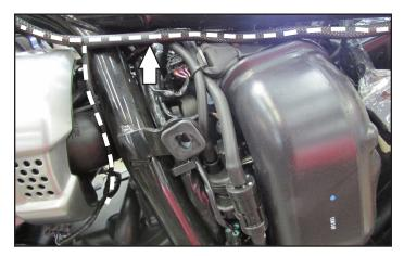
8 Unplug the stock Throttle Position Sensor connector.
