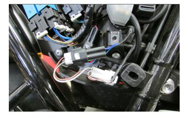
6 Plug the PC6 in-line of the stock CPS and wiring harness.
