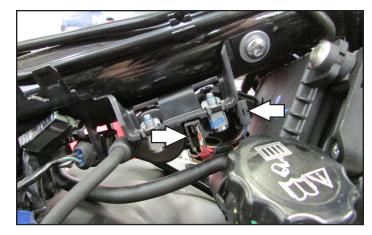
20 Plug the PC6 in-line of the stock wiring harness and #1 ignition coil.
