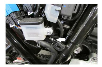
5 Locate the stock Crank Position Sensor on the right hand side of the motorcycle and unplug it.
