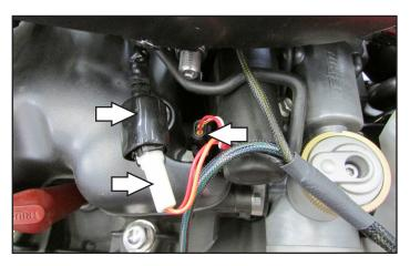
11 Plug the PC6 in-line of stock injector and wiring harness.
