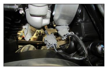
10 Unplug the stock wiring harness from both fuel injectors.
