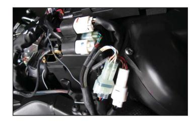
Using the supplied Posi-7 tap attach the GREY wire of the PC6 harness to the stock WHITE wire of the small ECU plug.
