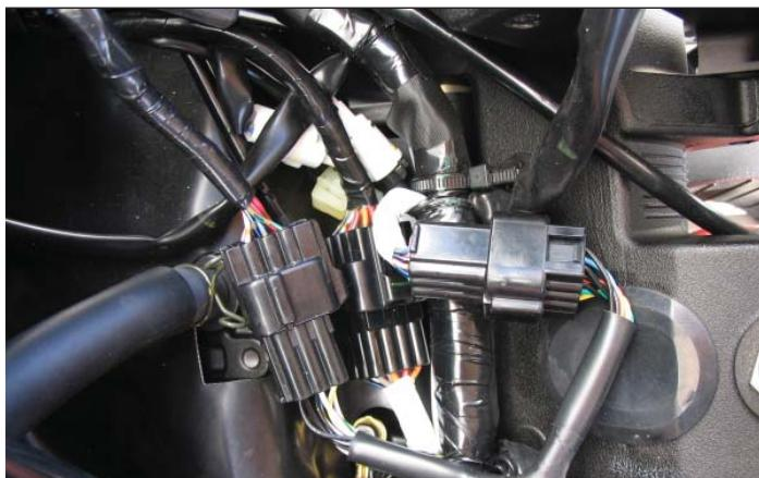
8 Attach the ground wire from the PC6 to the negative (-) terminal of the bike's battery as shown.
