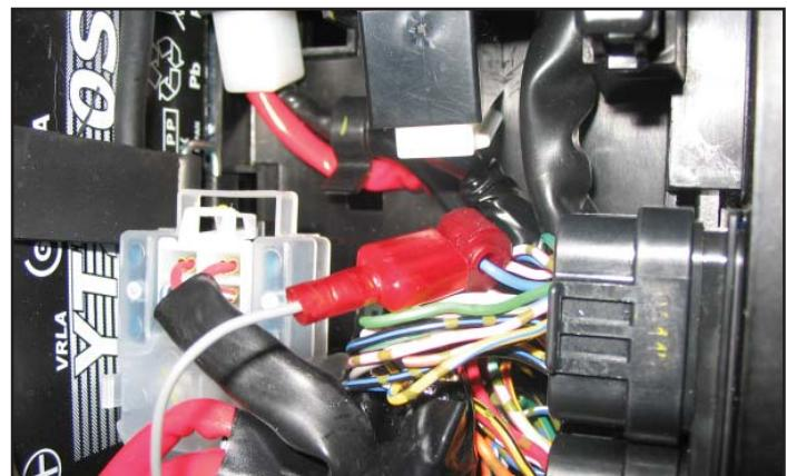
10 Using the supplied Velcro, secure the PC6 in the tail section of the bike as shown.
