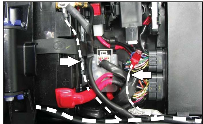
9 Using the supplied posi-tap, attach the GREY wire of the PC6 to the BLUE wire on the ECU.
