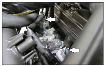
8 Plug the PC6 wiring harness in-line of the Fuel Injectors and the stock wiring harness.
