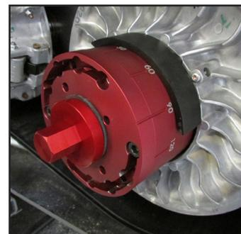
Loosen the compression tool enough to remove the compression block. Fully tighten the compression tool so that you can install the drive belt. Remove the compression tool. Keep this tool with you as it will be needed to change the belt.
