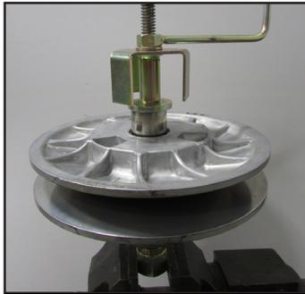
Take notice of the arrow marks on each sheave. It is best to make marks on the edge of each sheave with a marker for ease of reassembly. Slide the secondary assembly over the compression tool and tighten the tool down.
