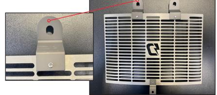
Install the assembled radiator shield onto the motorcycle using the stock hardware that was removed previously.
