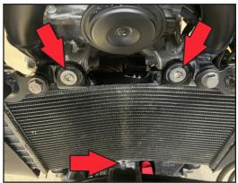
Install the brackets onto the Dynojet Radiator shield. The top LH bracket has a punch mark on the backside for reference.
