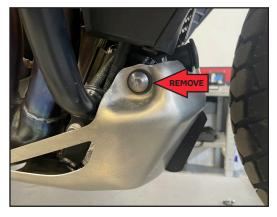
Using a T30 torx remove the 3 bolts holding the radiator in place.
