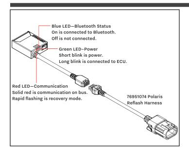
Thank you for purchasing the Power Vision 4 (PV4) from Dynojet Research. The Power Vision 4 is the most flexible and powerful flash tuning device in the world. The Power Vision 4 uses reflash technology to change the parameters inside the stock Engine Control Unit (ECU) that affects the way the engine will run.
