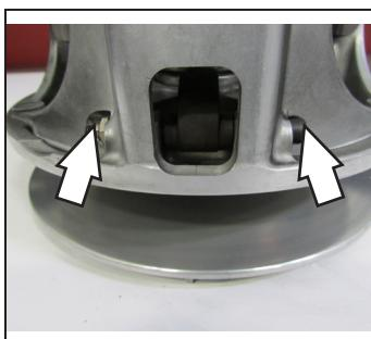
Remove the clutch arms using 3/8" socket and 1/8" allen key. Install the Dynojet clutch arms with the proper amount of weight. Refer to chart on page 2. Install the Dynojet primary spring and reinstall the spring cover. Tighten the 6mm bolts evenly to 9 ft-lb (12 Nm).
