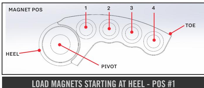
LOAD MAGNETS PER THE TABLE ABOVE. MAKE SURE EACH CLUTCH ARM IS LOADED WITH THE SAME AMOUNT OF WEIGHT.
