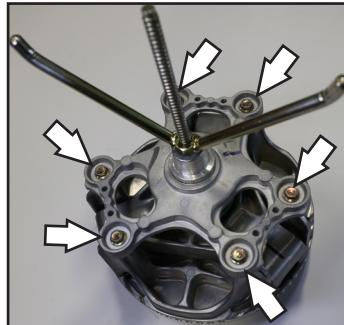
Remove the stock clutch arms by removing the pivot bolt for each arm. Lift the spider up slightly to allow room to remove the arms. Load the Dynojet clutch arms with the appropriate amount of weights from page 2. Install the
