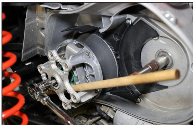
Use a wooden dowel to hold the primary assembly from rotating. Make sure the dowel does not touch the machined tower surface of the drive clutch. Remove the retaining bolt with a T60 torx.
