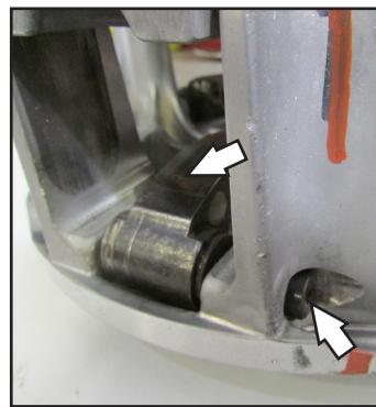
Dynojet clutch arms. Make sure to inspect the rollers for wear along with the pivot bolts before reassembly. Install the Dynojet GREEN primary spring and reassemble the primary. Align the marks on each part and torque the clutch cover bolts to 15 ft-lbs. Install the primary assembly and torque the drive clutch bolt to 125 ft-lbs.
