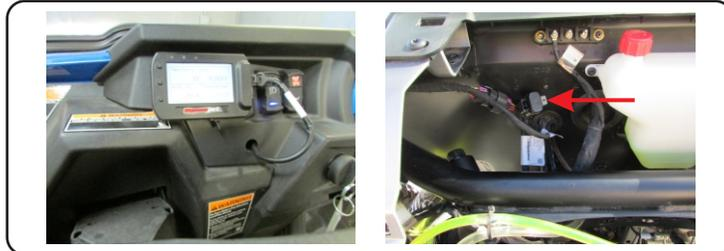
1. Secure the PVCX to the vehicle using the supplied Velcro or a suitable mount using the standard AMP mounting holes on the back of the PVCX. Make sure the PVCX will not interfere with the operation and steering of the vehicle.
