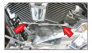
Thread the supplied Dynojet shift rod into the female end of the Dynojet shift sensor and tighten. Put the stock lock nuts from the stock shift rod onto the Dynojet shift rod/ shift sensor assembly.
