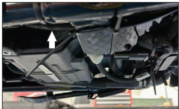
16 Unplug the stock Crank Position Sensor.
