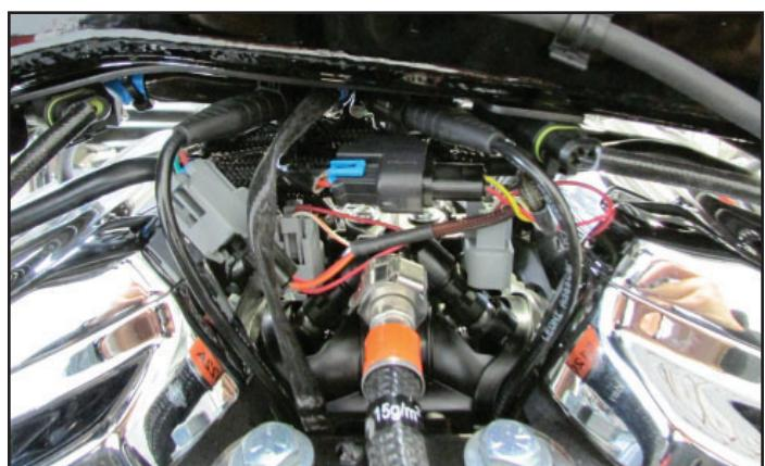
11 Unplug the stock wiring harness from the Throttle Position Sensor.
