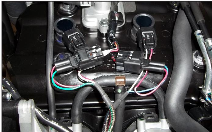
10 Connect the PC6 wiring harness in-line of the stock ignition coils and wiring harness.
