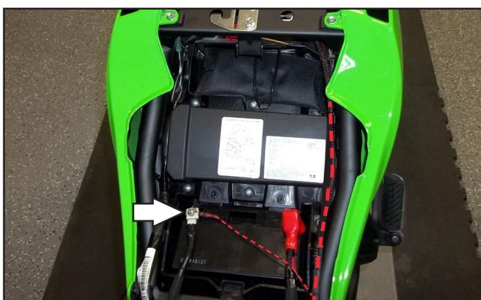
13 Attach the PC6 ground wire to the negative side of the battery.
