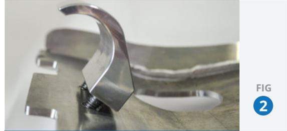
Note: leave the clamp a loose and angled as shown to ease installation
