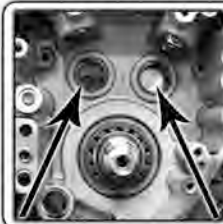
Replace inner cam bearings use the proper tools
