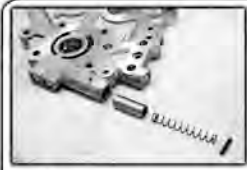
Inspect pressure relief valve
