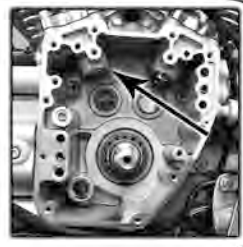
Verify Intake lobes of camshafts clear engine case Crank bearing boss & lifter bosses
