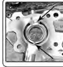
Inspect camplate for scoring, if scoring is present replace camplate. Scoring will effect oil psi & oil scavenging
