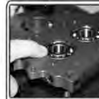
Verify bearings are flush with camplate
