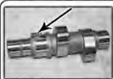
Install cam keys - use arbor press or vise with soft jaws
