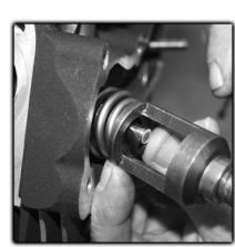
FEULING recommends the use a seal installer to prevent seal damage. Install spring, retainer & locks.
