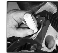
FEULING recommends the use a seal installer to prevent seal damage. Install spring, retainer & locks.
