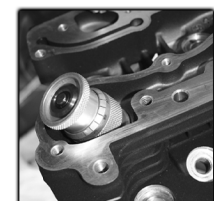
Measure spring installed height and seal to retainer clearance. Proper clearance from coil bind is critical.
