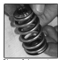
Clean & Inspect new springs & hardware
