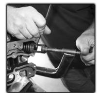
Remove original valve springs & hardware
