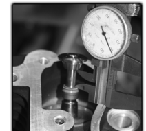
Measure spring installed height and seal to retainer clearance. Proper clearance from coil bind is critical.
