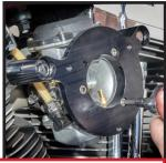
Insert backing plate bolts to help center backing plate & breather bolt holes. Final torque breather bolts to 22-24 ft/lbs. Final torque backing plate bolts to 36-60 in/lbs (Carburetor) 72 in/lbs (EFI)
