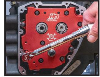
Install camplate bolts finger tight. Use moly lube/engine oil on under head flange & threads.
