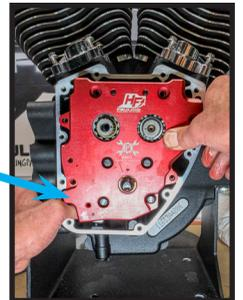
**NOTE:** If unable to get assembly fully seated, the thinner pressure gear is most likely mis-aligned.
