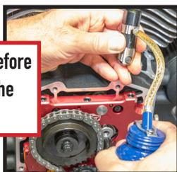
Install lifters into engine case with anti-rotation pins.
