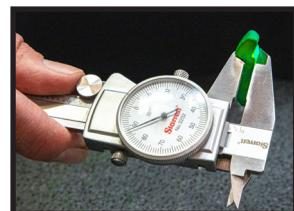
Measure thickness of clay after cycling engine.
