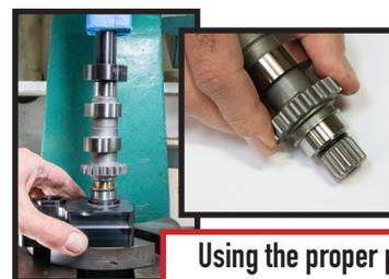
Using the proper press tools and lube install the race onto the camshaft.
