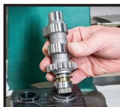
Install race from new rear cam bearing as the race is matched to the bearing.
