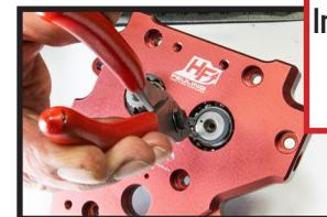
Install retaining ring on front camshaft.
