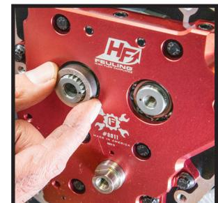
**21.** Using a sprocket locking tool install the sprocket retention hardware. Apply a small amount of moly lube to the under head flange of the bolts & Loctite 263 (Red) to the threads. Both bolts should be initially torqued to **15 ft/lbs**. & then loosened one full rotation. Final torque the pinion shaft bolt to **24 ft/lbs**. & the rear sprocket bolt to **34 ft/lbs**.
