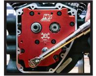
**20.** Install sprockets, lining up the timing marks. Check sprocket alignment with a straight edge, use correct thrust washer thickness to achieve proper sprocket alignment. See Feuling #8040 for spacer thickness selection/options. Sprocket alignment is critical for wear & longevity of tensioner pad.
