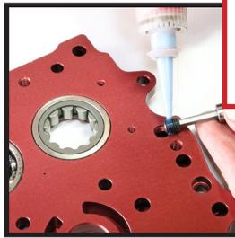
If installing the 1/16" boss plug, apply Loctite & torque to **55-60 in/lbs.**
