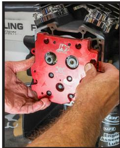
Using your thumb to press pump inward can aid in installation.
