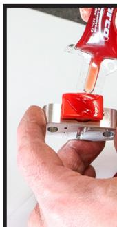
Lube inner tensioner pad, chain, & inner bore of tensioner housing.
