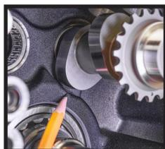
Verify camshaft lobe rotating clearance to engine case.
