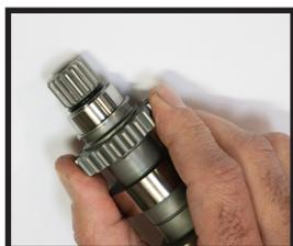
Remove existing rear cam race from outer journal. Use a separator in a press or with a standard puller.
