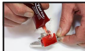
Install outer tensioner. Use assembly lube on the tensioner pad & chain. Verify pad is square to chain & not cocked.
