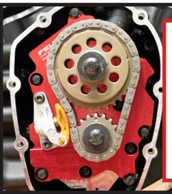
Step Torque cam & crank bolts first to 15 ft/lbs. loosen then re-step torque up to a final torque:
