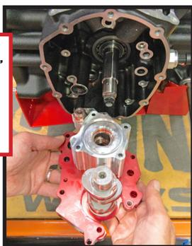
Use your thumb or finger to help push the oil pump into the scavenge port of engine case.
