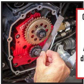
Check sprocket alignment with a straight edge.
