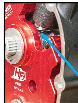
**20.** Install lifter feed holes facing each other, we also recommended rotating the engine over with the lifter 'cuffs' finger tight to center the holders on the lifters before final torque.
