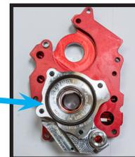
If desired, install O-ring/seal from factory pump. Remove O-ring/seal from factory cover and install into Feuling back cover.
