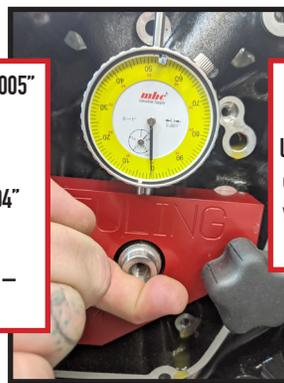
Measure crank bearing play by lifting up on the tip of the pinion shaft with dial indicator in place.
