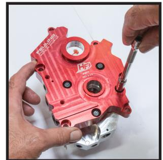
**NOTE:** DO NOT USE LOCTITE ON OIL PUMP OR CAMPLATE BOLTS, use moly lube paste, assembly lube or oil on bolt threads & underhead flange. Loctite will interfere with the stack up clearance of the oil pump & can cause sealing issues with camplate to engine case.
