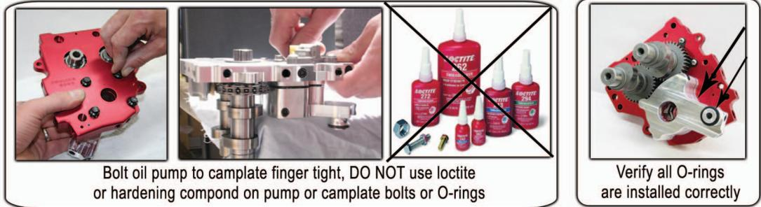
15. Verify camshaft lobes DO NOT interfere with the engine case. Install new O-rings into proper location on crankcase.
