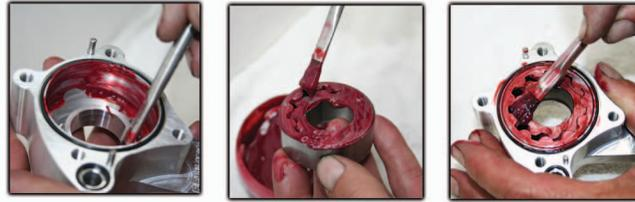
13. Bolt the complete Feuling Oil Pump to the camplate **finger tight**, with the pressure housing of the pump facing the camplate. **DO NOT** use loctite or any type of hardening compound on oil pump or camplate bolts or O-rings, the compound will interfere with stack up tolerance. Grease can be used to hold O-rings in place and moly lube or engine oil should be used on all bolts and underhead flanges
