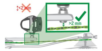
**9** If the pedal rubs the chain, add one washer (included) between the spindle and the crank arm to increase clearance.
