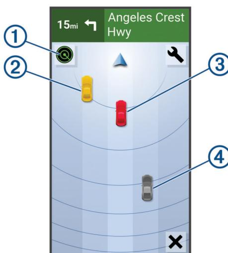
The vehicle positions change color based on threat level. The status icon **1** indicates the radar sensor status. A yellow vehicle **2** indicates a vehicle is approaching in your blind spot to the left or right of your motorcycle. A red vehicle **3** indicates a vehicle is approaching rapidly or presents a danger. The rear alert light flashes red three times when this occurs. A gray vehicle **4** indicates a vehicle is approaching from a distance.
