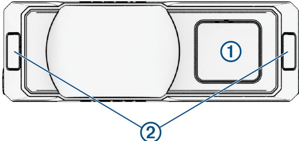
**NOTE:** The rear-facing red light ① may be oriented to the left or right, depending on which fit is most suitable for your motorcycle.
