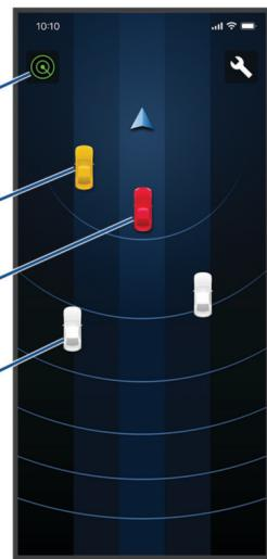
The status icon ① indicates the radar sensor status. The vehicle positions change color based on threat level. A yellow vehicle ② indicates a vehicle is approaching in your blind spot to the left or right of your motorcycle. A red vehicle ③ indicates a vehicle is approaching rapidly or presents a danger. The rear alert light flashes red three times when this occurs. A gray vehicle ④ indicates a vehicle is approaching from a distance.
