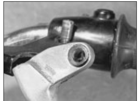
3.2b . . . and withdraw lever, noting shim (where fitted)
