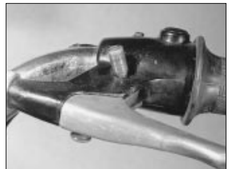
3.2a Remove handlebar lever pivot screw . . .
