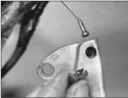
3.2c Disengage cable inner from slotted trunnion
