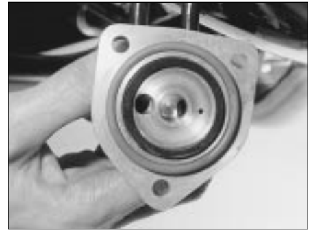
1.22 Ensure seals are correctly installed before refitting adapter
