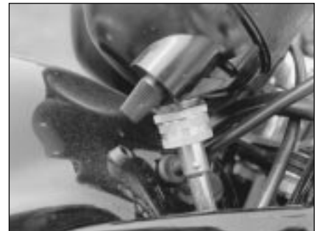
3.11 Instrument drive cables are retained by knurled rings at their upper ends
