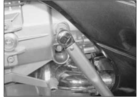
10.3b . . . and tighten it to the specified torque setting
