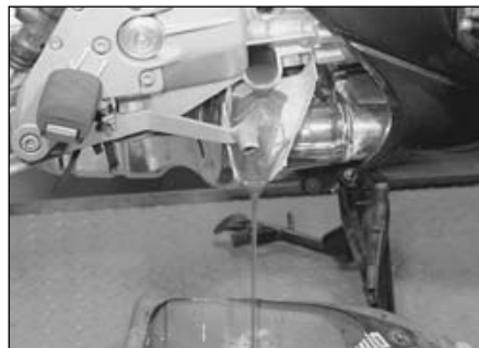
13.2b . . . and allow the oil to drain completely – note the cardboard chute
