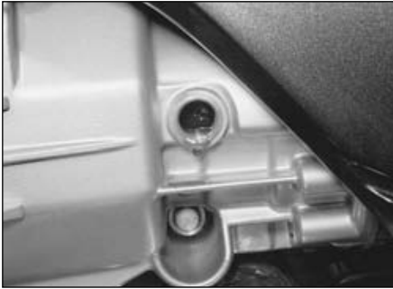
10.2 The gearbox oil should be level with the lower edge of the filler hole
