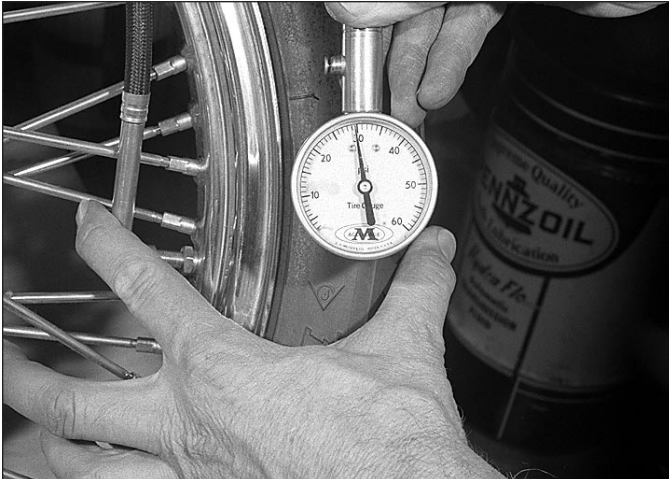
8.4 Check tire pressures with an accurate gauge
