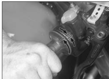
8.3a Check for a small amount of freeplay in the throttle twistgrip
