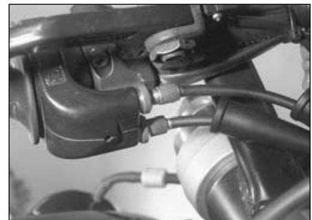
8.3b Cable adjuster(s) is/are located below twistgrip housing – carburettor model shown
