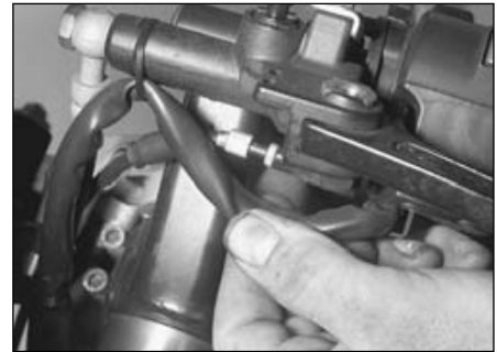
8.10 Choke cable adjuster is located below left-hand handlebar switch housing
