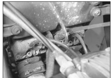
9.3b A long handled Phillips screwdriver is necessary for idle speed adjustment
