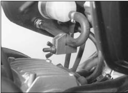
7.13 Hose clamp can be used on the fuel inlet hose to prevent fuel flow
