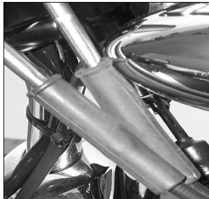
13.13a Slide back the rubber boots for access to the throttle cable adjusters
