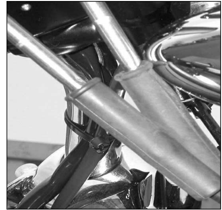
18.13a Slide back the rubber boots for access to the throttle cable adjusters
