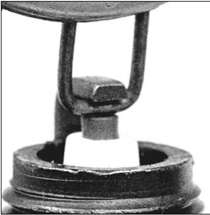
20.6a Spark plug manufacturers recommend using a wire-type gauge when checking the gap - if the wire doesn't slide between the electrodes with a slight drag, adjustment is required
