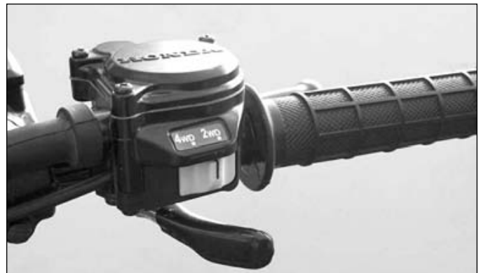
11.2 Measure throttle freeplay at the lever
