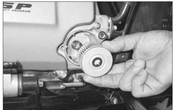
14.6c . . . remove the filter and spring and wipe the remaining oil out of the filter housing; be sure the filter element's OUT SIDE mark faces outward on installation
