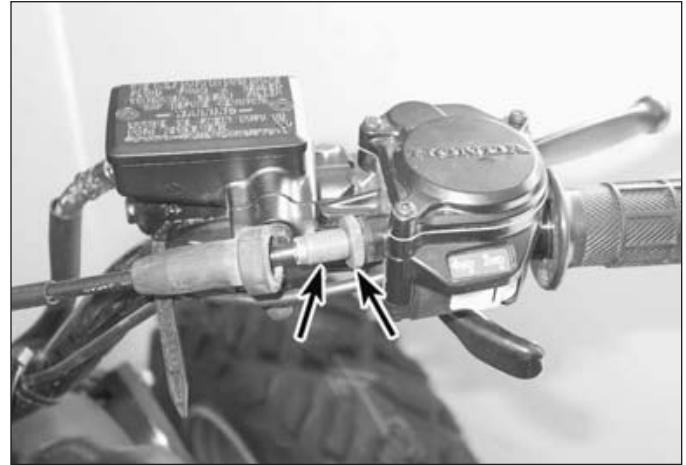
11.3 Loosen the lockwheel (right arrow) and turn the adjuster wheel (left arrow) to make fine adjustments in throttle freeplay
