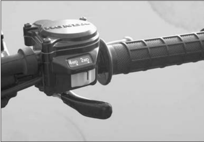
11.2 Measure throttle freeplay at the lever
