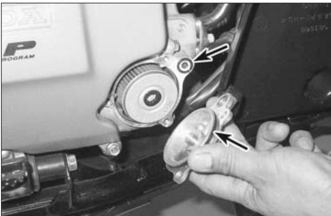
14.6b . . . pull off the cover and note the O-ring locations (arrows) . . .
