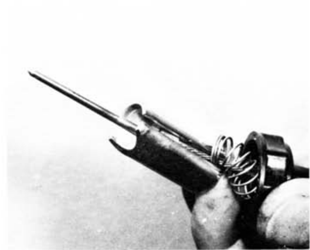
7.4 Remove throttle valve assembly from the cable
