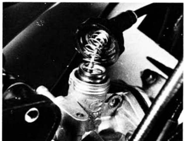
6.2 Unscrew carburettor top to release throttle valve assembly
