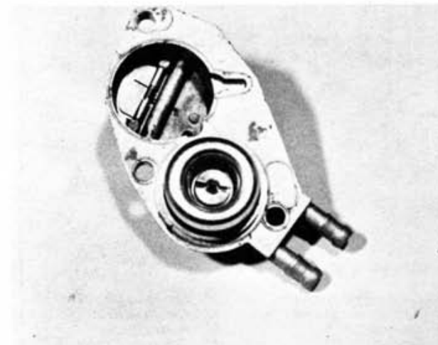
8.3b ... and unscrew the float valve seat ...
