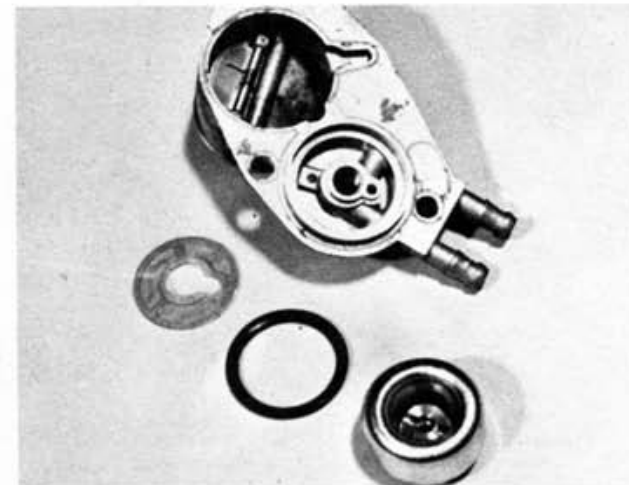
8.3c ... and remove the petrol filter
