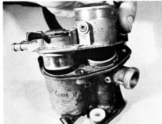
8.3a Remove the screws and the float chamber top ...
