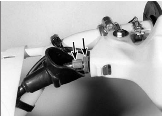
7.2 Loosen the lockwheel (right arrow) and turn the adjuster wheel (left arrow) to make fine adjustments in clutch lever freeplay
