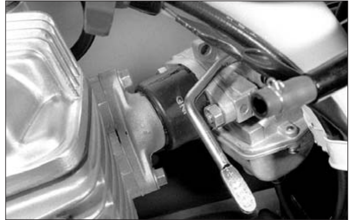
9.1 Move the choke lever back and forth and check for smooth operation
