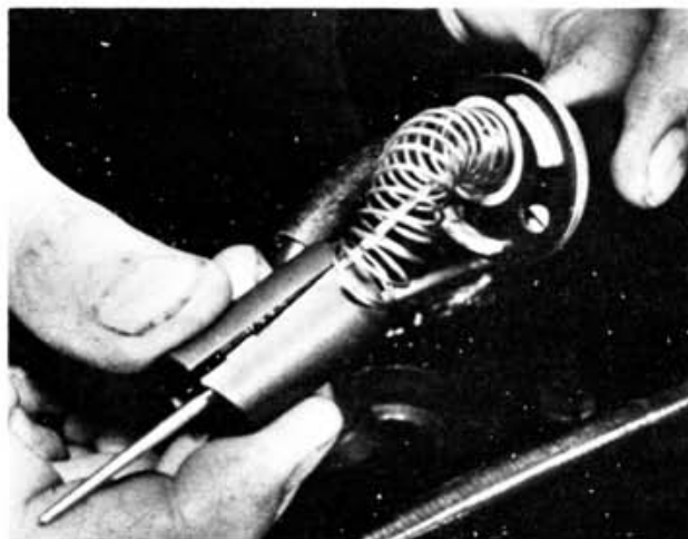
5.6a If necessary, the throttle valve may be detached from the cable
