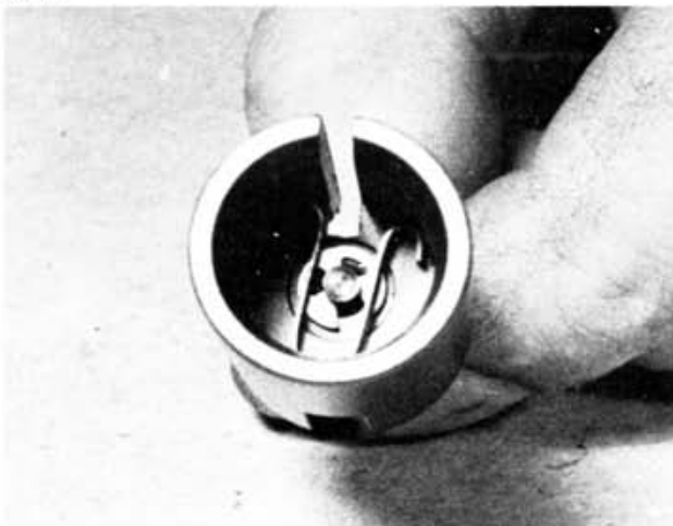
5.6c ... locates within the valve and retains the needle spring clip
