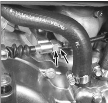
5.4 To make major clutch cable adjustments on a CR80R, loosen the locknut (right arrow) and turn the adjusting nut (left arrow)
