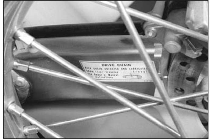
2.1 Decals on the motorcycle include maintenance information such as drive chain adjustment
