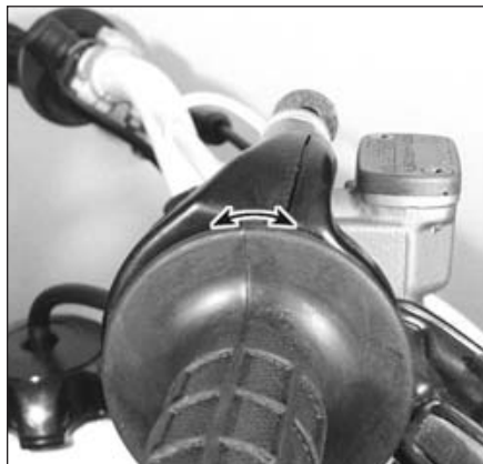
4.2 Measure throttle freeplay at the grip
