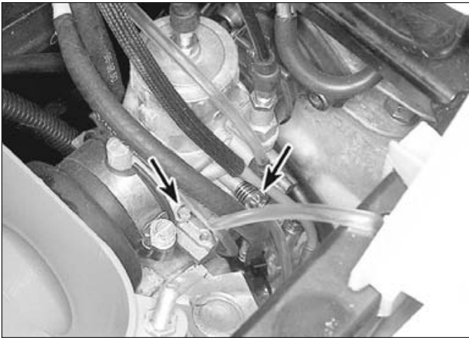
12.3a Two-stroke pilot screw (left arrow) and throttle stop screw (right arrow)
