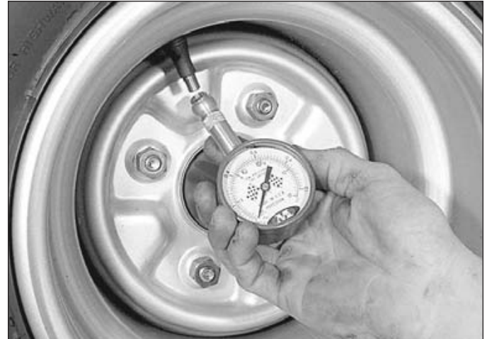
10.4 Check tire pressure with a gauge that will read accurately at the low pressures used in ATV tires
