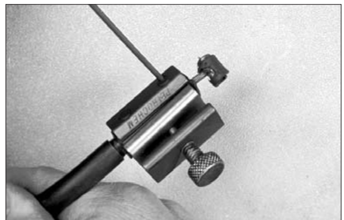
10.3 Lubricating a cable with a pressure lube adapter (make sure the tool seats around the inner cable)
