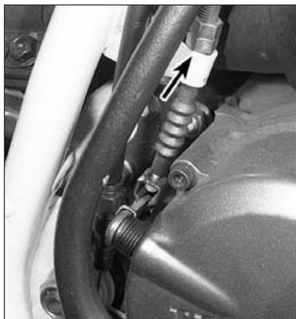
7.4a Major adjustments are made at the lower adjuster; it's behind the clutch cover on XR250L and XR250R models . . .
