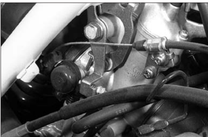
9.2 The choke cable is attached to this bracket on the carburetor
