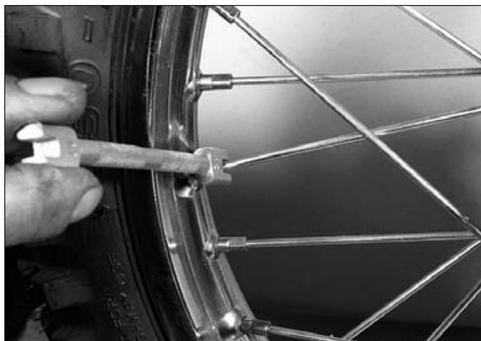
6.5 Make sure the spokes are tight, but don't overtighten them
