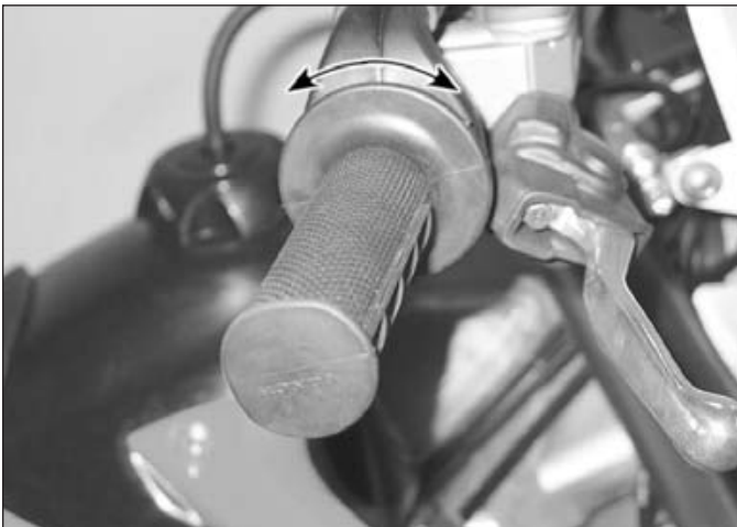
8.2 Measure throttle freeplay at the grip
