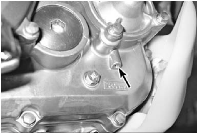
7.5a If coolant is leaking from the small hole under the water pump (arrow), it's time for a new water pump seal. This is a CRF250X (CRF250R similar) . . .
