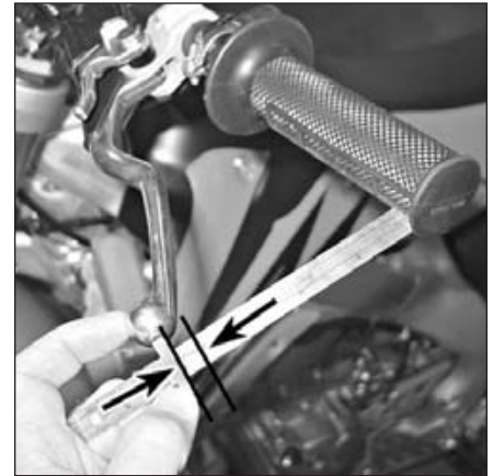
9.1 Measure clutch freeplay at the lever tip
