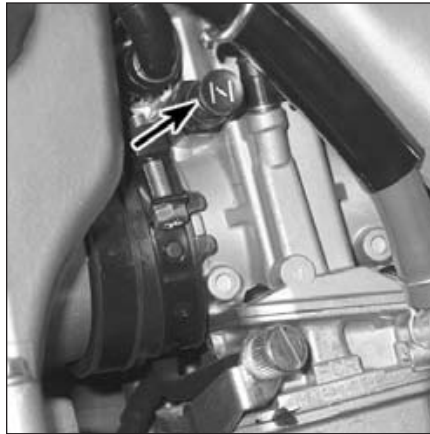
8.6 The choke knob should click when pulled out and pushed in
