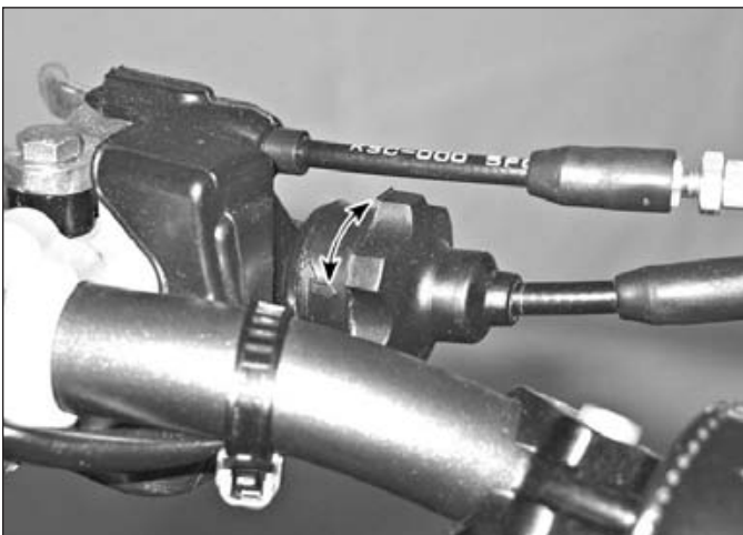
9.2 Turning the thumbwheel toward you (when sitting on the seat) will increase clutch lever freeplay; turning it away from you will decrease freeplay
