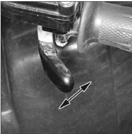
8.3 Check throttle lever freeplay at the lever tip
