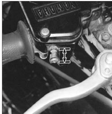
8.7 Measure limiter screw length from the throttle housing to the underside of the screw head
