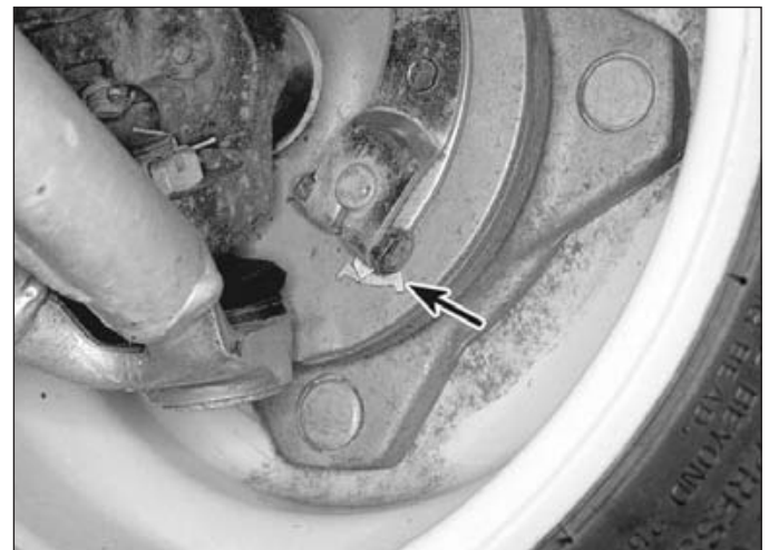
11.6 If the pointer aligns with the forward mark when the front brakes are applied (arrow), it's time to replace the front brake shoes
