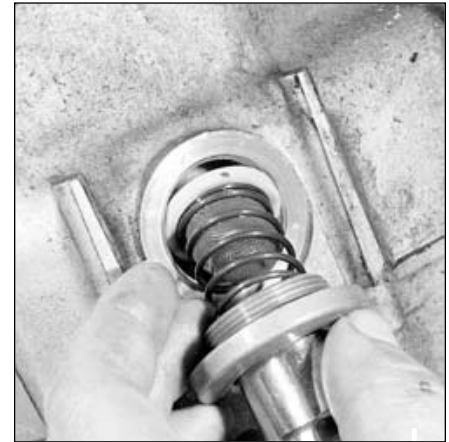
13.6a Unscrew the oil drain plug and remove the O-ring, spring and strainer
