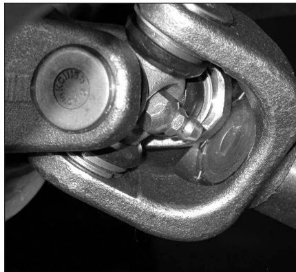
12.7a Driveshafts on some models have a grease fitting at each end
