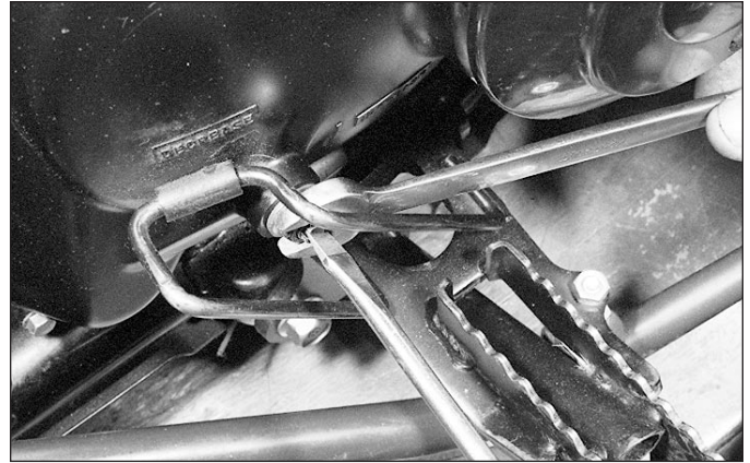
9.2 Loosen the locknut, then hold it with a wrench while you turn the adjusting screw
