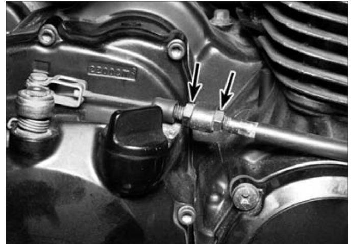
11.3 To adjust the clutch cable at the engine, loosen the nuts (arrows), turn them to move the cable housing, then tighten the nuts
