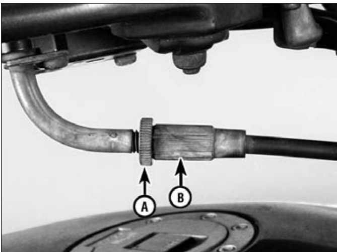
10.6 To adjust throttle freeplay, loosen the lock wheel (A), turn the adjuster (B), then tighten the lock wheel
