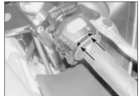
7.4 Measure the amount of freeplay in the throttle as shown
