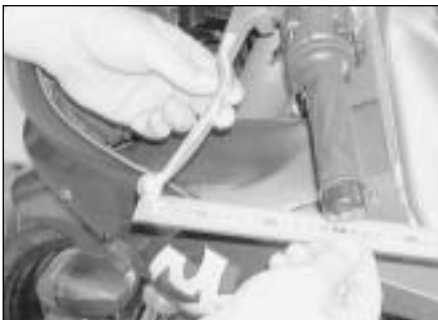
8.5 Check the amount of freeplay in the cable as shown
