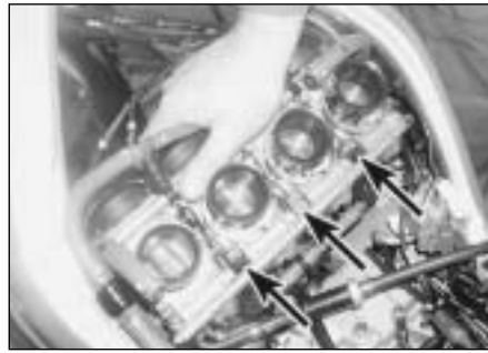
5.8 The synchronisation screws are located in the linkage between the carburettors
