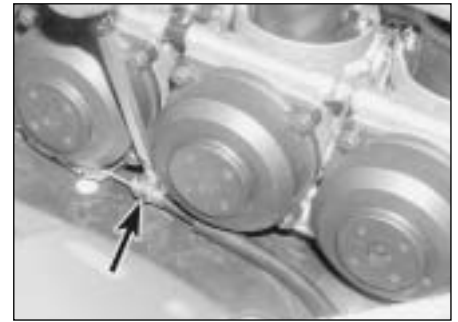
7.13 Choke cable clamp (arrowed) at carburettor end
