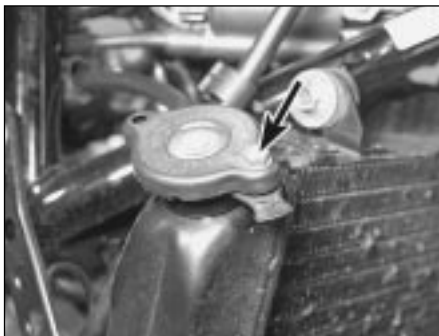
16.6a On TRX models, remove the pressure cap security bolt (arrowed)
