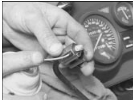
18.3a Lubricating a cable with a cable oiler clamp
