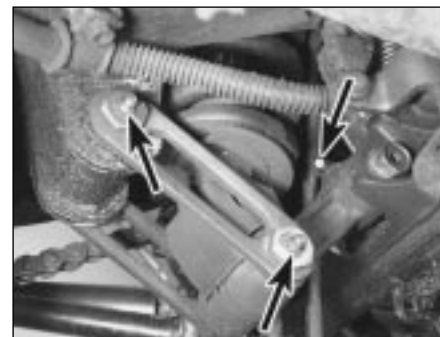
19.1 Apply grease to the nipples on the suspension linkage (arrowed) and to the nipple on the swingarm pivot
