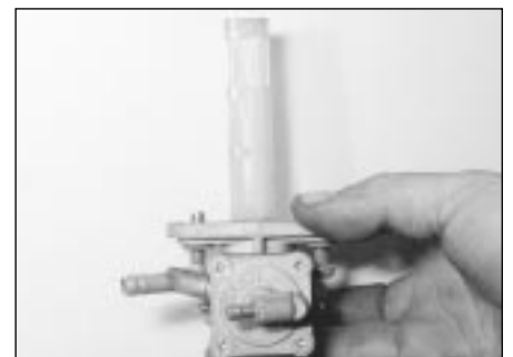
6.5 The fuel tap incorporates a gauze type filter
