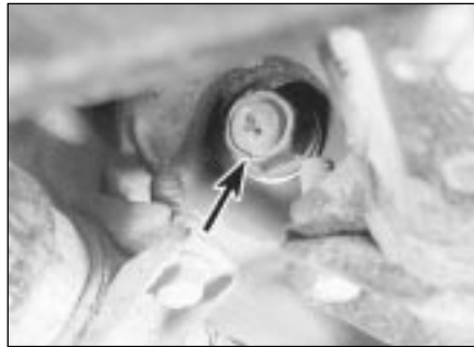
7.4 The oil drain plug (arrow) is located at the front of the sump
