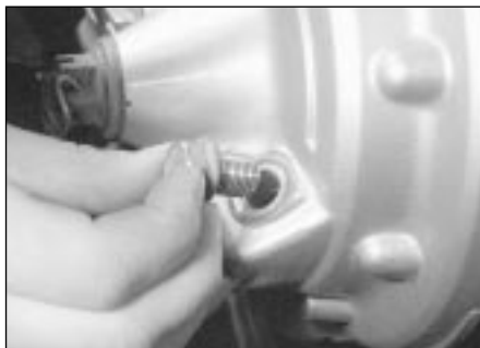
8.2a Unscrew the oil filler cap from the final drive housing . . .
