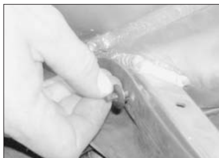
18.7a Fit the trim clip into its socket . . .
