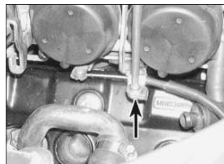
18.10 Slacken the clamp screw (arrowed) and slide the cable into the clamp a little
