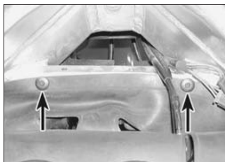
18.5a Release the trim clips (arrowed) . . .
