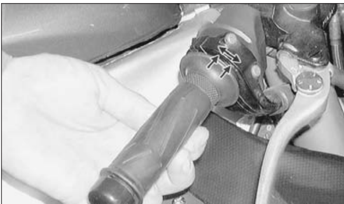
18.3 Measure the amount of freeplay in the throttle as shown
