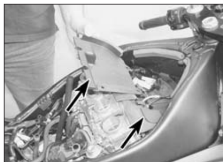
18.5d Remove the ignition coil plate in two sections (arrowed)
