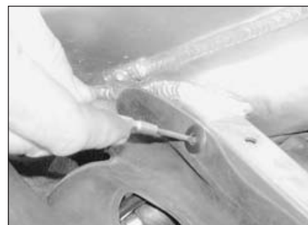
18.5c Push the centre into the body and remove the clip
