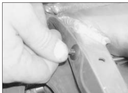
18.7b . . . and push the centre into the body to secure it
