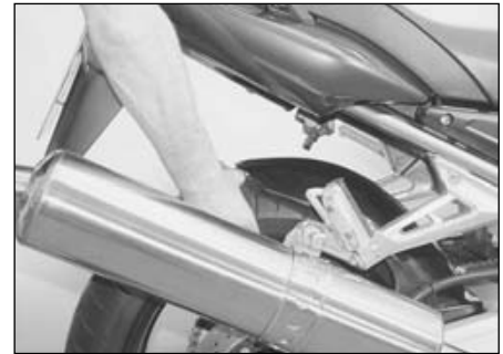
19.8 Checking for play in the suspension linkage bearings
