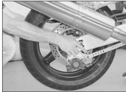
19.7 Checking for play in the swingarm bearings
