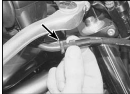
17.4 Slacken the locking (arrowed) and turn the adjuster as required
