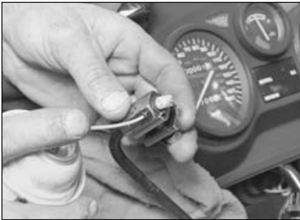
18.3 Lubricating a cable with a pressure lubricator. Make sure the tool seals around the inner cable
