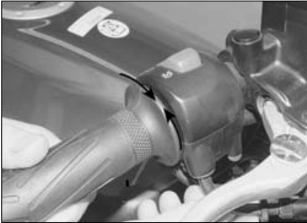
17.3 Measure the amount of freeplay in the throttle as shown
