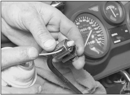
6.4a Lubricating a cable with a pressure adapter. Ensure the tool seals around the inner cable
