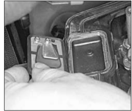
14.3b Lift the valve out of the cylinder head for inspection
