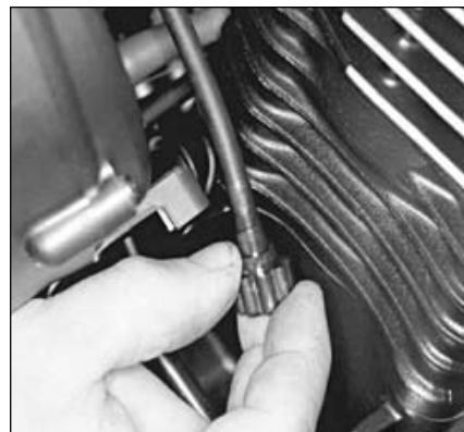
17.3b The Vulcan 800 idle speed knob is at the end of this stalk
