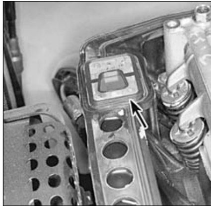
14.3a On Vulcan 800 models, remove the valve covers for access to the air suction valves (arrow)
